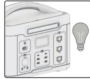
When all ports are off the Arc12 will automatically shut off after 30 seconds.
